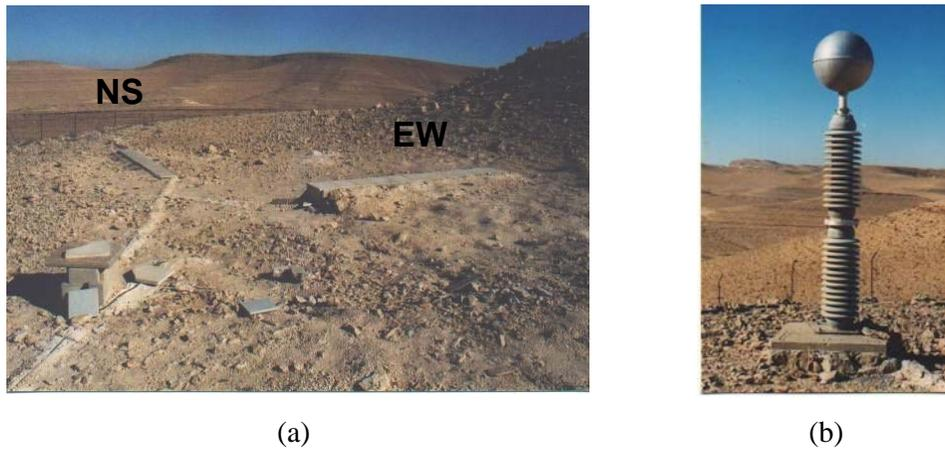
Figure 2: ELF sensors- (a) Magnetic field coils and (b) Electric field ball antenna.
